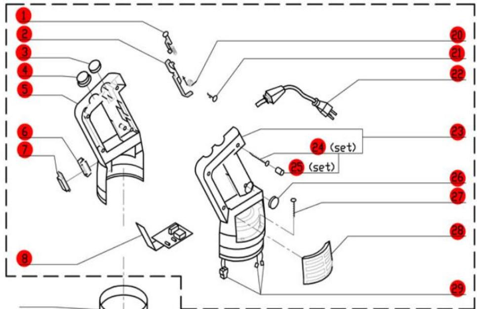
If replacing internal parts within dashed lines, order a set of replacement screw caps, part # MP29544.
